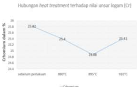
Gambar 3. Grafik Hubungan Heat Treatment Terhadap Nilai Unsur Logam Chromium (Cr)
