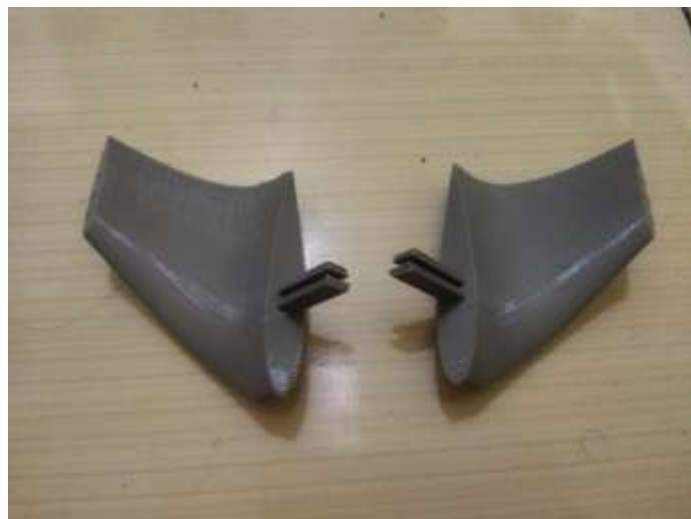
Gambar 2. Model Turbin Angin Darrieus Dua Bilah Hasil 3D Printing
