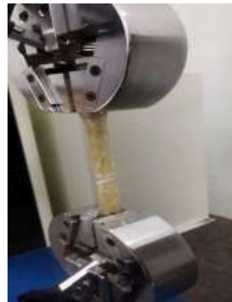
Gambar 2. Proses uji tarik
