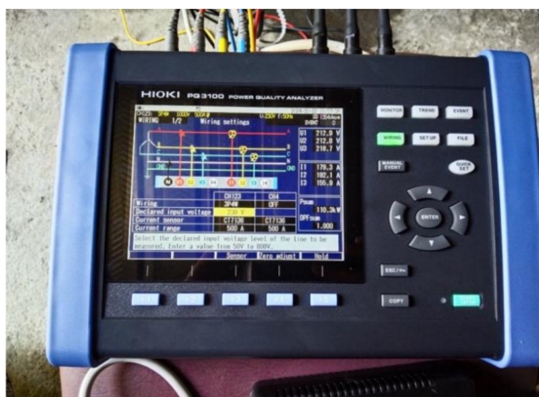
Gambar 4. Power Quality Analyzer 3100 Merek Hioki
