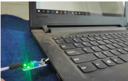
Gambar 3.3. Pengujian Sensor Infrared
