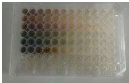
Figure 1. MIC measurement on 96 well plate on 6 samples and 1 control sample. Extracted pigments obstructed effective reading for a quantitative determination of MIC.
